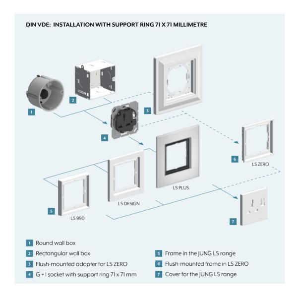
If the G + I socket is installed in a wall box according to DIN VDE, combinations in up to five-gang frames are possible. This results in numerous function possibilities.
